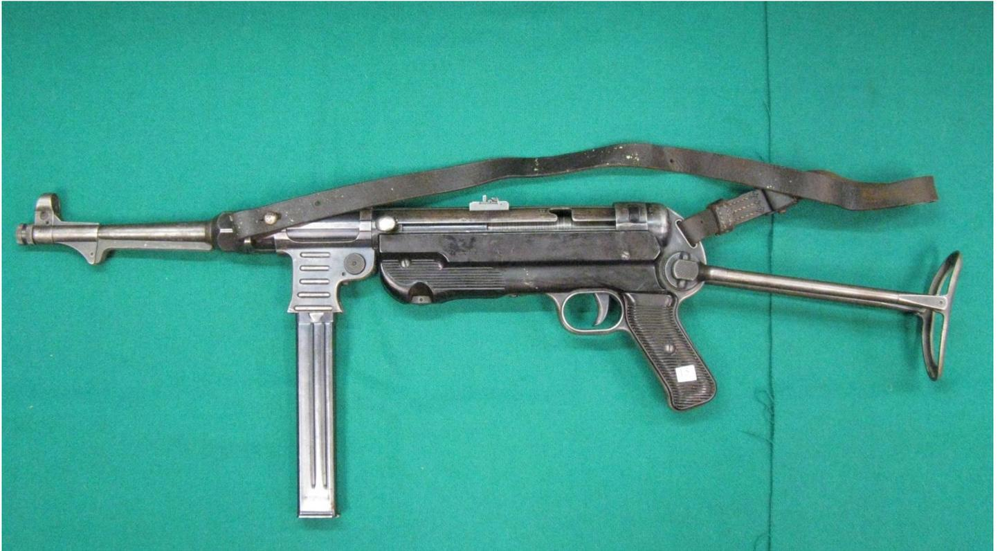
The Schmeisser MP 40 machine pistol or sub-machine gun was one of the outstanding German weapons of WWII. A development from early German sub-machine guns, it was one of the first to employ extensive sheet metal stampings, ridiculed at first by other countries, it proved its' worth in the beginning of WWII and led to the adoption in other countries of similar guns, such as the British Sten and the U. S. N 3.
